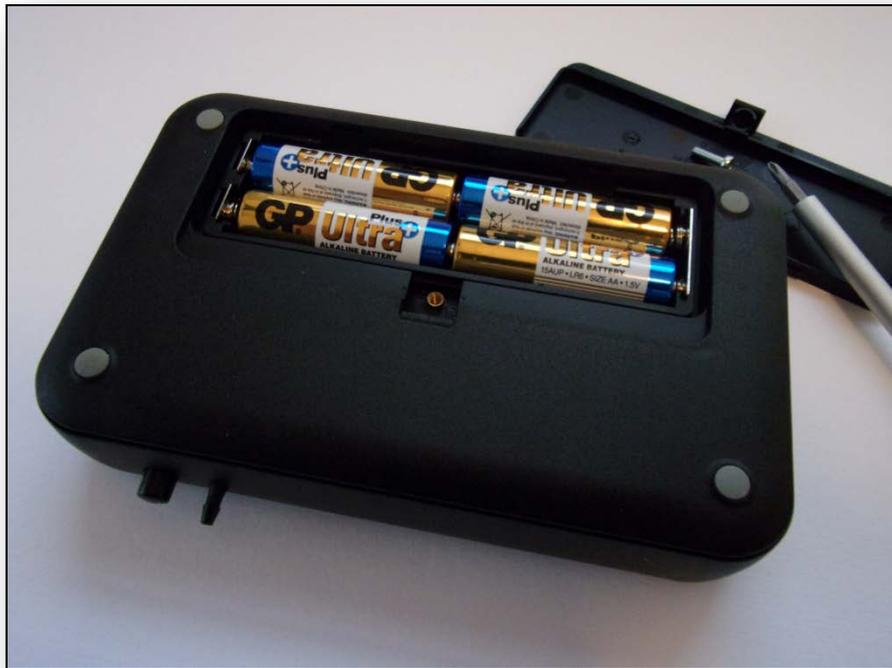
Photo 1.2.1.1: the leak tester, battery compartment
