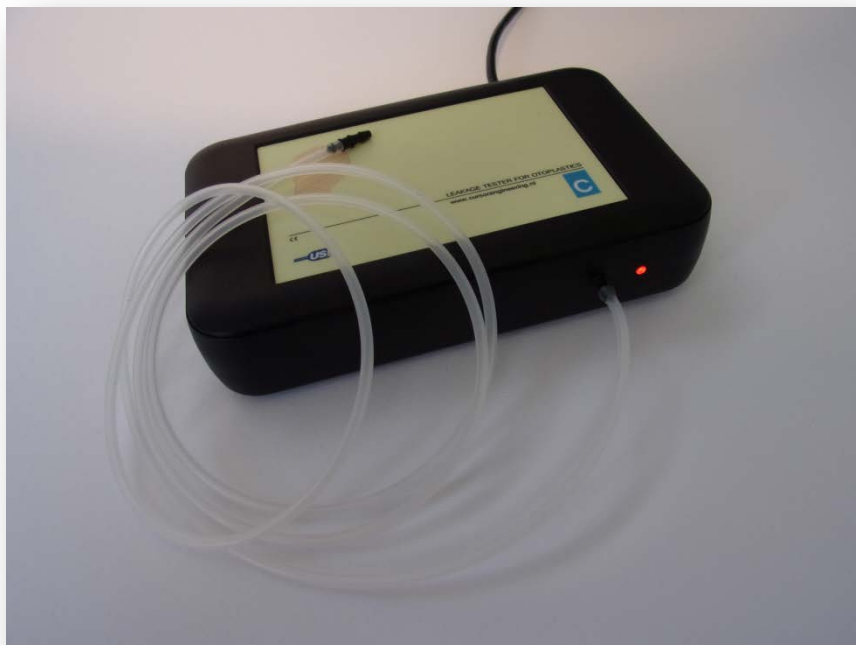
Photo 1.1.1: the USB leakage tester, front and silicon hose with standard adapter
