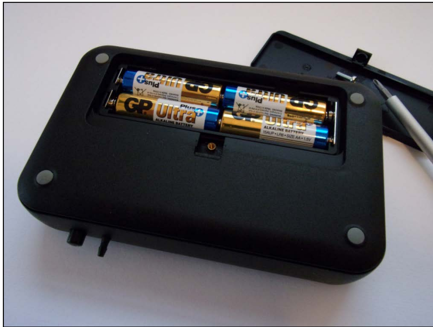
Photo 1.2.1.1: the leak tester, battery compartment
